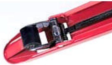
6.5" wide forks have welded steel entry glides, polyurethane load rollers, and an additional exit roller for ease of exiting the pallet
